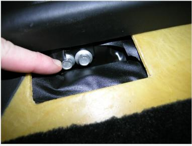
Now your door panel should be pretty bare with the exception of the door handle itself. Under the handle there is a small Philips head screw that has to be removed. The pic shows the silver colored screw. Unscrew and gently pull the handle TOWARDS you. It seats on the assembly with notches and may be tight at first. Do not try to turn it. It pulls off straight towards you. When reinstalling the handle it will only slide on one way because of the notches.
