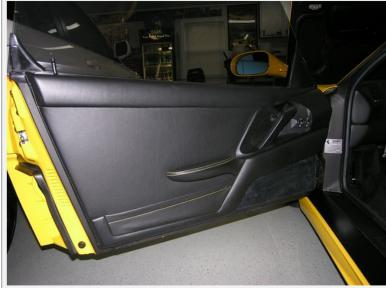
Remove lock knob by unscrewing it. It is threaded almost the entire length of the knob so it takes quite a few turns to get it off-
