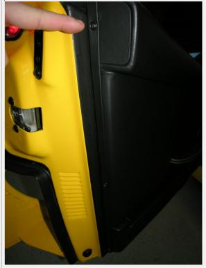
Now locate the mirror trim piece towards the front of the door panel, up near the outside mirror. This metal triangle shaped piece is held on by 2 Philips head screws. Remove both screws and gently pull the trim piece off.
