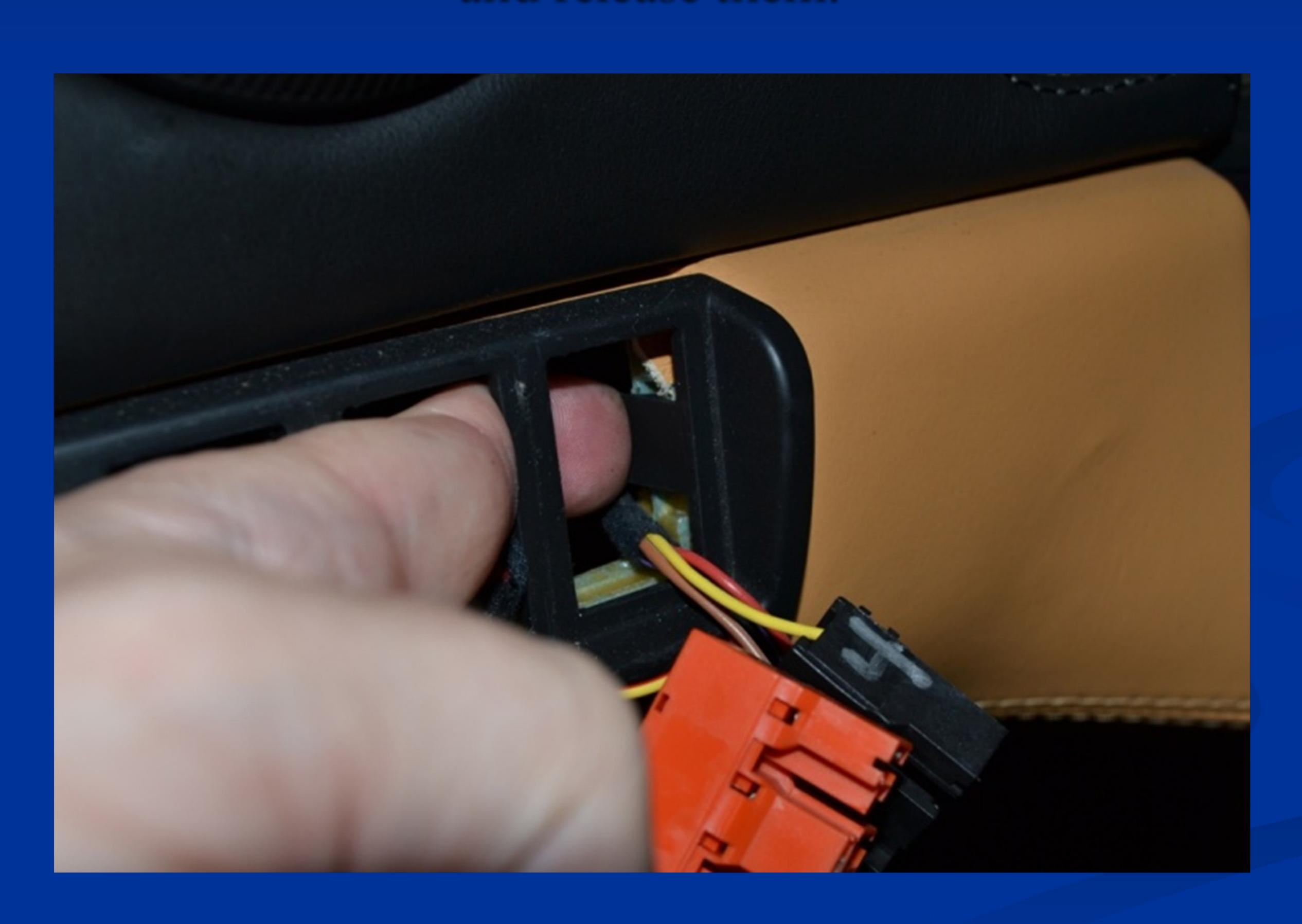
Push the switch connectors back thru there holes in the trim and gently pull the entire trim forward.
