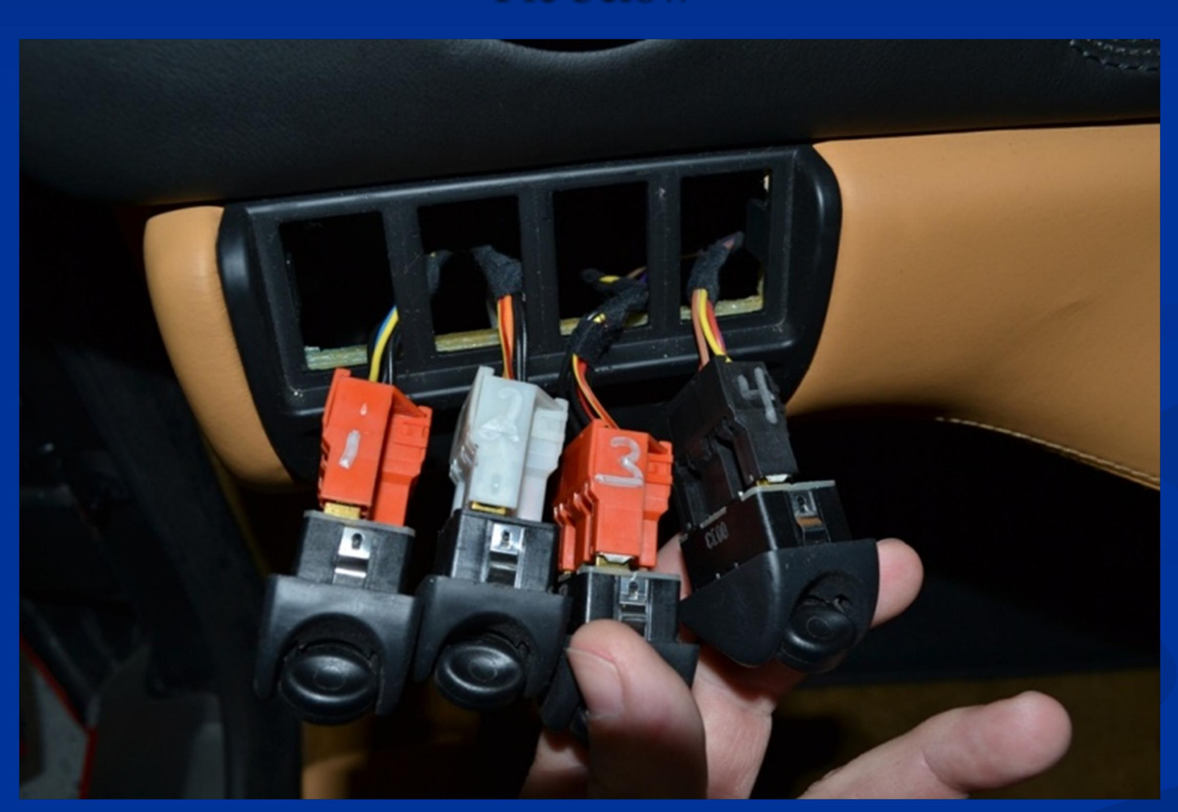
Now pull each connector off of each switch and set the switches aside. If you look inside the trim you will see a small tab on both sides. This tab needs to be lightly pulled inward to release the trim from the dash. The pic below shows the tab I am referring to. There also may be two similar tabs at the inside top of trim. You can easily feel for them and release them.
