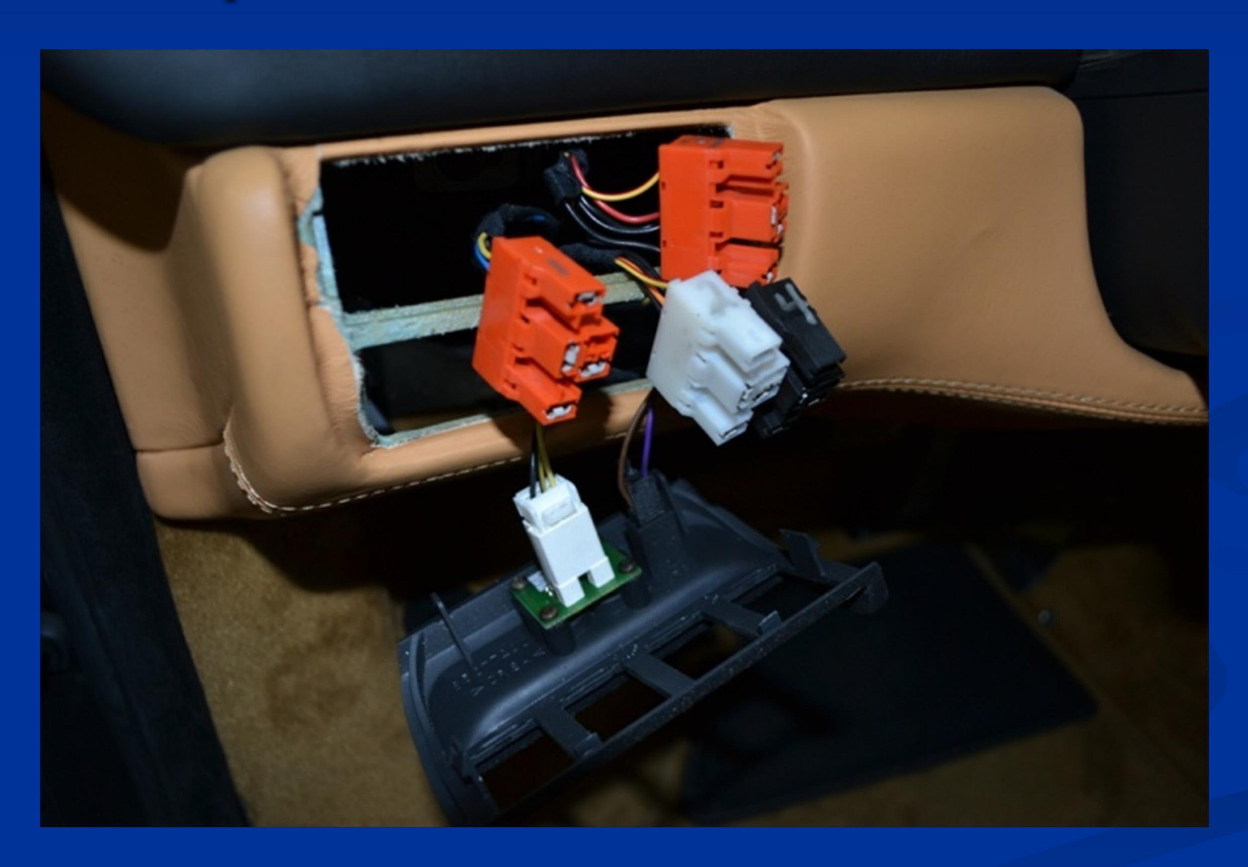
Unclip the white connector and the alarm light connector.
